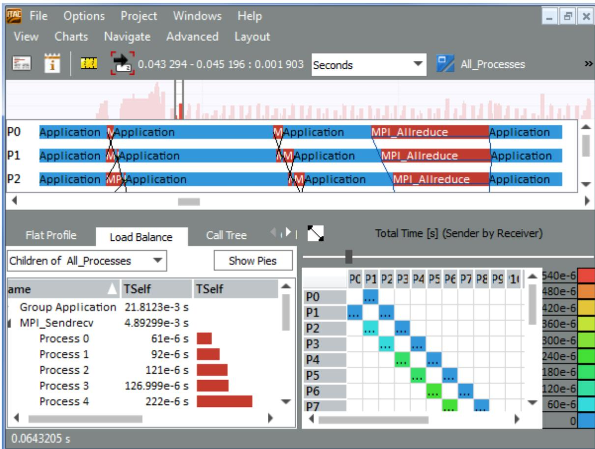
In the Load Balance tab, expand MPI\_Sendrecv and MPI\_Allreduce. The Load Balancing indicates that the time spent in MPI\_Sendrecv increases with the process number, while the time for MPI\_Allreduce decreases.
