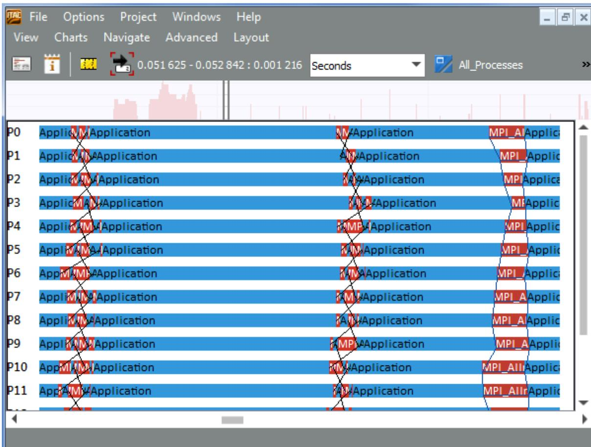
Since `poisson_sendrecv.single.stf` is a striking example of serialization, almost all of the Intel® Trace Analyzer charts show this interesting pattern. But in the real-world cases, it may be necessary to formulate a hypothesis regarding how the program should behave and to check this hypothesis using the most suitable chart.
