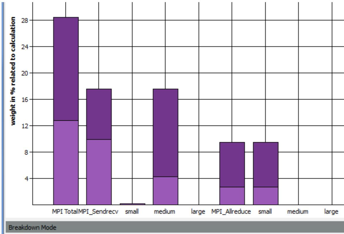
You can see that `MPI_Sendrecv` is the most time-consuming function. The imbalance weight is displayed in pink color and comprises about 10% for the `MPI_Sendrecv` function. This is the time the processes spend waiting for each other.
