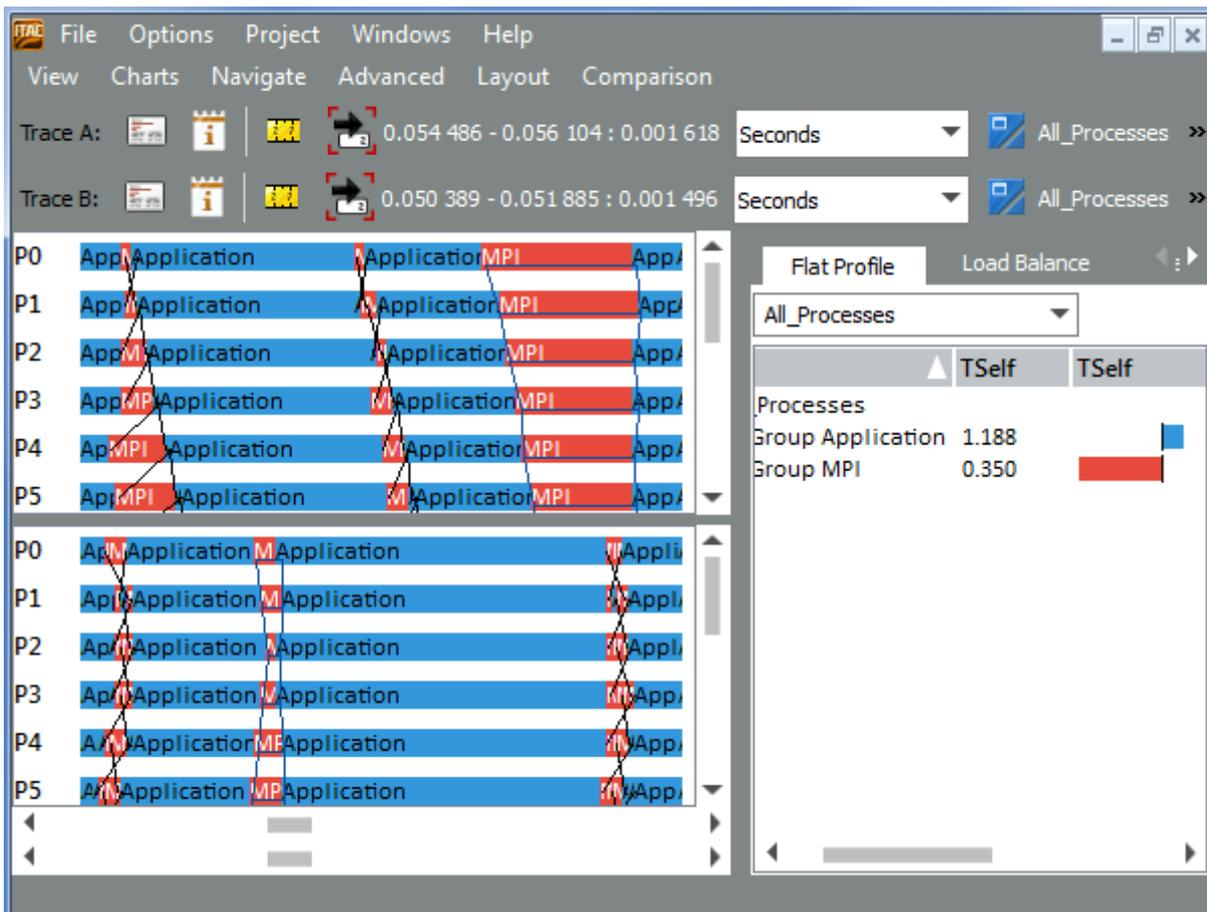
In the Comparison View, you can see that using non-blocking communication helps to remove serialization and decrease the time of communication of processes.
