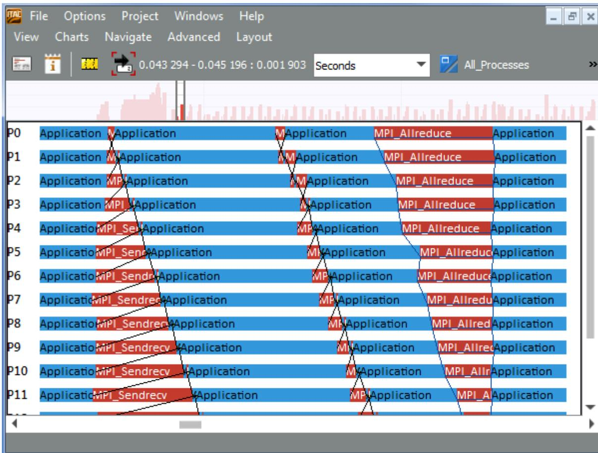
After ungrouping the MPI functions, you see that the processes communicate with their direct neighbors using MPI\_Sendrecv at the start of the iteration.
